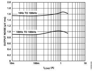
Figure 28. RMS Output Noise vs. Load Current (ILOAD)
