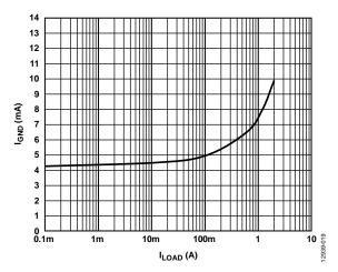
Figure 19. Ground Current ( $I_{GND}$ ) vs. Load Current ( $I_{LOAD}$ ),  $V_{OUT} = 1.2 \text{ V}$
