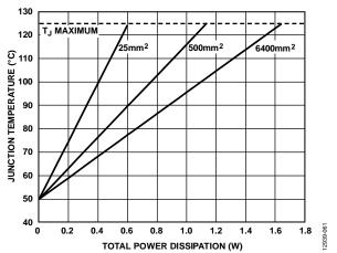
Figure 59. Junction Temperature vs. Total Power Dissipation for the 8-Lead SOIC,  $T_A = 50^{\circ}$ C
