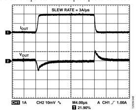
Figure 44. Output Transient Response,  $V_{OUT}$  = 3.3 V,  $C_{OUT}$  = 10  $\mu$ F, Channel 1 = Load Current, Channel 2 =  $V_{OUT}$
