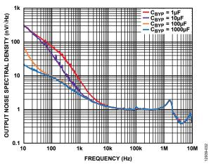
Figure 30. Output Noise Spectral Density vs. Frequency at Various Values of C<sub>BYP</sub>
