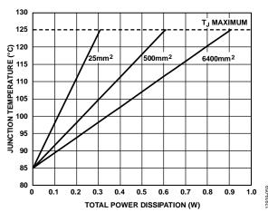
Figure 57. Junction Temperature vs. Total Power Dissipation for the 10-Lead LFCSP,  $T_A = 85^{\circ}C$
