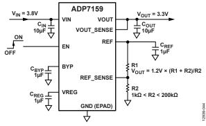
Figure 42. Typical Adjustable Output Voltage Application Schematic
