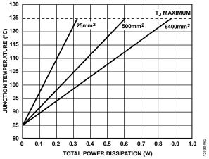
Figure 60. Junction Temperature vs. Total Power Dissipation for the 8-Lead SOIC,  $T_A = 85^{\circ}C$
