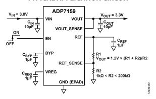
Figure 1. Regulated 3.3 V Output from 3.8 V Input
