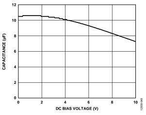
Figure 47. Capacitance vs. DC Bias Voltage
