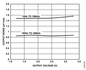
Figure 29. RMS Output Noise vs. Output Voltage
