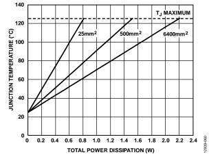
Figure 58. Junction Temperature vs. Total Power Dissipation for the 8-Lead SOIC,  $T_A = 25^{\circ}C$
