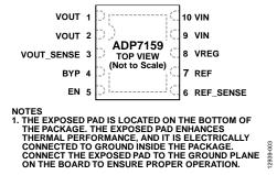
Figure 3. 10-Lead LFCSP Pin Configuration
