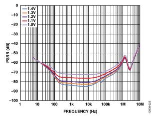
Figure 25. Power Supply Rejection Ratio (PSRR) vs. Frequency at Various Headroom Voltages,  $V_{OUT}$  = 1.2 V, 2 A Load
