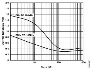
Figure 45. RMS Output Noise vs. Bypass Capacitance (CBYP)
