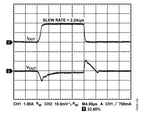
Figure 34. Load Transient Response,  $I_{LOAD} = 100$  mA to 2 A,  $V_{OUT} = 3.3$  V,  $V_{IN} = 4.0$  V,  $C_{OUT} = 22$   $\mu$ F, Channel  $1 = I_{OUT}$ , Channel  $2 = V_{OUT}$
