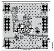
Figure 63. Sample 10-Lead LFCSP PCB Layout
