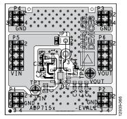
Figure 64. Sample 8-Lead SOIC PCB Layout
