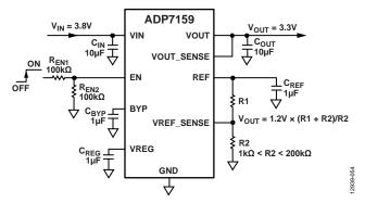
Figure 52. Typical EN Pin Voltage Divider
