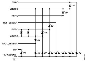
Figure 43. Simplified ESD Protection Block Diagram
