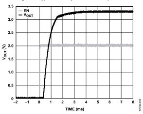
Figure 50. Typical  $V_{OUT}$  Response to EN Pin Operation ( $V_{EN}$ ),  $V_{OUT} = 3.3 \ V$ ,  $V_{IN} = 5 \ V$ ,  $C_{BYP} = 1 \ \mu F$
