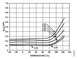
Figure 5. Shutdown Current (I<sub>IN-SD</sub>) vs. Temperature at Various Input Voltages (V<sub>IN</sub>), V<sub>OUT</sub> = 1.8V
