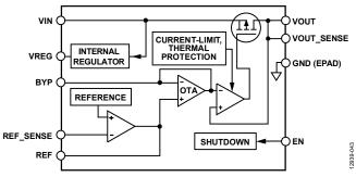
Figure 41. Simplified Internal Block Diagram
